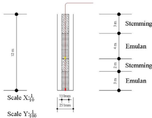
**Figure 6: Charge distribution and pre-splitting parameter in the hole for test3**
