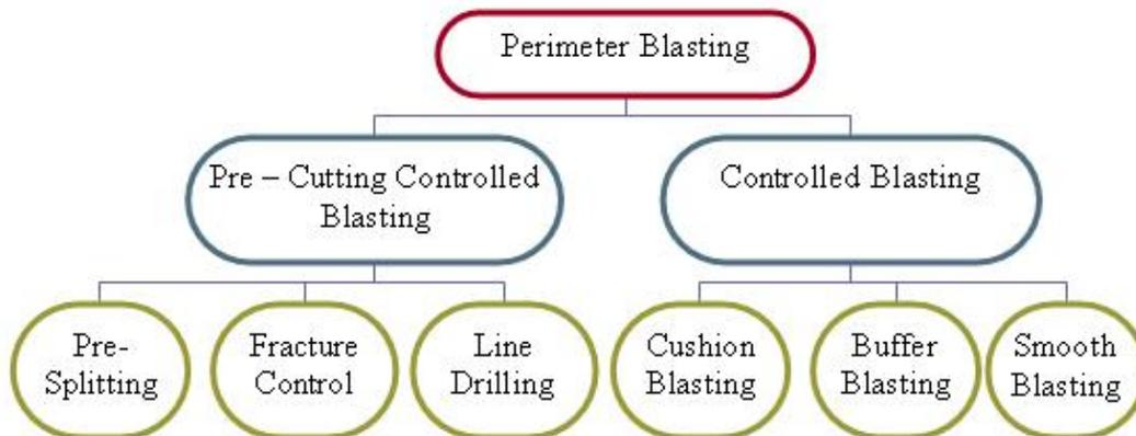
Figure 3: Perimeter blasting techniques
