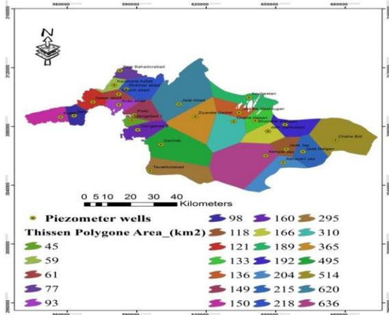
**Fig. 5.** Effective area of each piezometer well in Jaz Murian aquifer using the Thiessen method.
