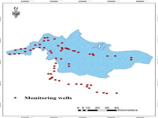
**Fig. 3.** Dispersion of monitoring wells which considered to interpolation of quality properties.
