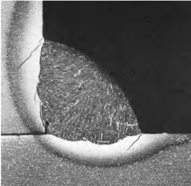
Figure 17.19 Hydrogen cracking in a fillet weld of 1040 steel (magnification 4.5 \times ). Courtesy of Buehler U.K., Ltd., Coventry, United Kingdom.
