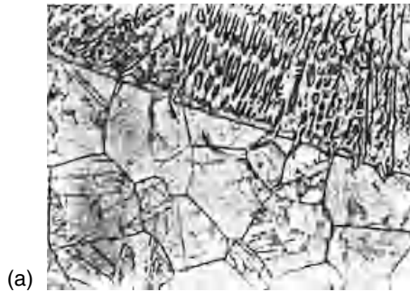
Figure 12.8 Schematic representation of constitutional liquation and formation of ghost GB network. Reprinted from Pepe and Savage (6). Courtesy of American Welding Society.
