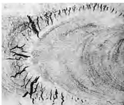
Figure 11.6 Solidification cracking tests: (a) Varestraint (15); (b) transverse Varestraint (16); (c) cracking in a ferritic stainless steel Varestraint specimen (17). (c) Reprinted from Krysiak et al. (17), courtesy of ASM International.
