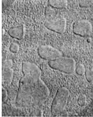
Figure 16.7 HAZ of Udimet 700 showing reprecipitation of fine \gamma' in region where coarse \gamma' begins to dissolve. Magnification 16,000 \times . Reprinted from Owczarski and Sullivan (13). Courtesy of American Welding Society.
