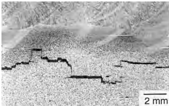
Figure 17.32 Lamellar tearing near a C–Mn steel weld. Reproduced by permission of TWI Ltd.
