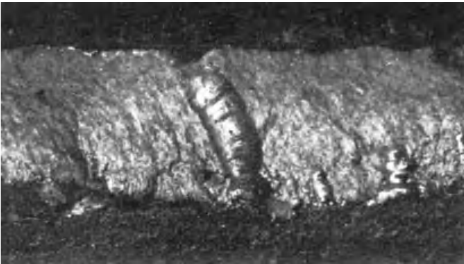
Figure 3.25 Wormhole porosity in weld metal. From Jackson (55).
