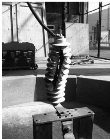
Fail in Pressure Relief Test at 20 kA/0.2sec on polymer housed distribution arrester
