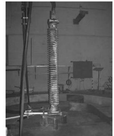
Successful Pressure Relief Test at 20 kA/0.2sec on polymer housed distribution arrester
