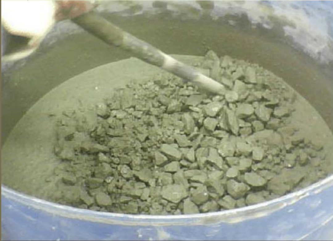
SEGREGATION IN CONCRETE
