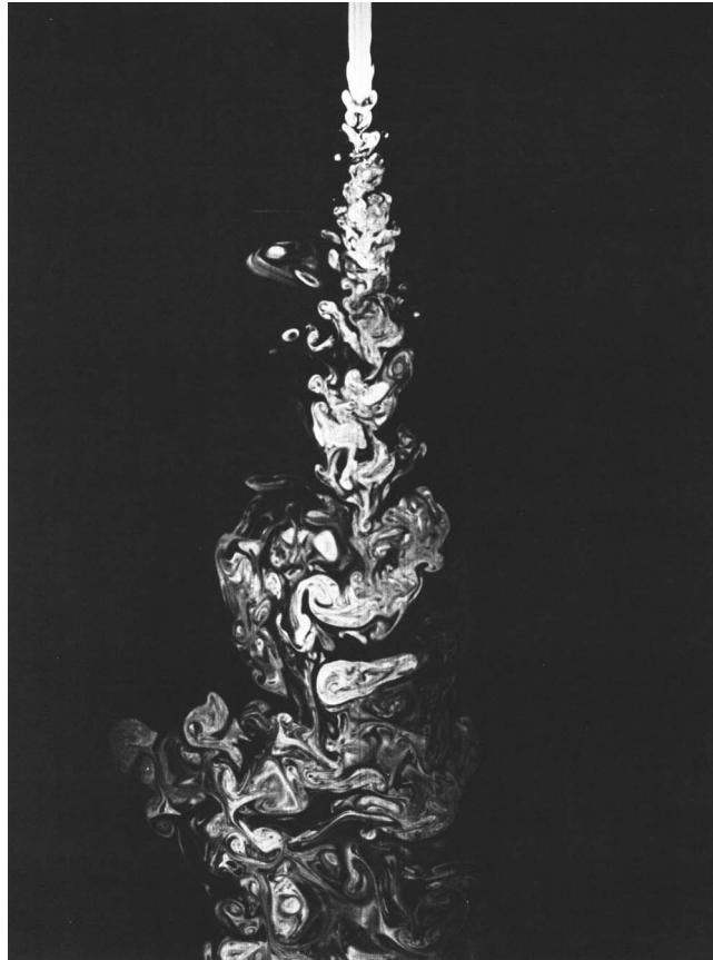
Figure 11.2 Turbulent jet issuing into a quiescent reservoir. The flow visualization technique makes visible the jet fluid in a plane containing the jet centerline.
