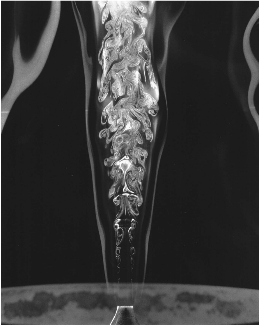
Figure 13.6 Visualization of nozzle-fluid flow patterns using reactive Mie scattering in methane–air jet flame ( v_e = 10 m/s, d_i = 10 mm). The total length of the image is approximately 20 nozzle-diameters. Near the nozzle, the flame zone resides just outside of the rollup of the nozzle shear layer. Near the top of the photograph, the flame zone interacts with the turbulent core. The visualization of an outer layer results from water vapor from the flame reacting with \text{TiCl}_4 vapor in the surrounding air flow.
