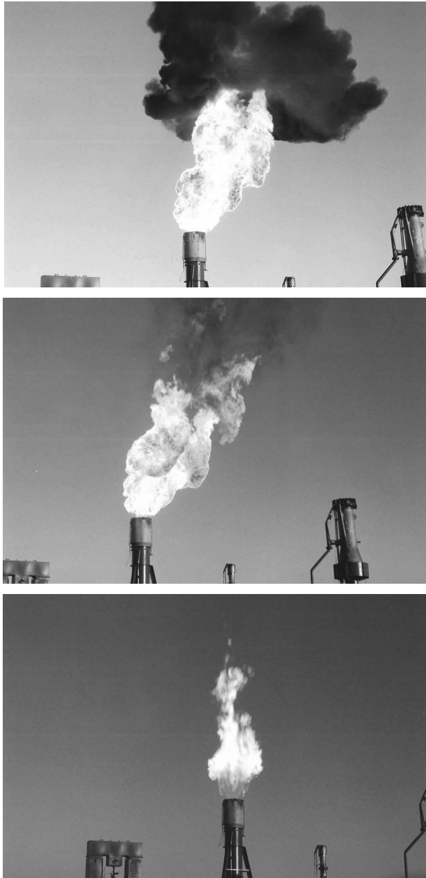
Figure 13.13 Flame radiation and soot are greatly reduced by injecting air during a flaring operation. Flaring of an unsaturated hydrocarbon shows extensive soot and visible radiation (top panel) before the air is injected. As the air blower comes up to speed, the visible soot diminishes (middle panel). At steady state, visible soot is eliminated and the radiation from the flame is greatly reduced by the injection of the air (bottom panel). | SOURCE: Photographs from Ref. [36] and used with permission of John Zink Company and CRC Press.
