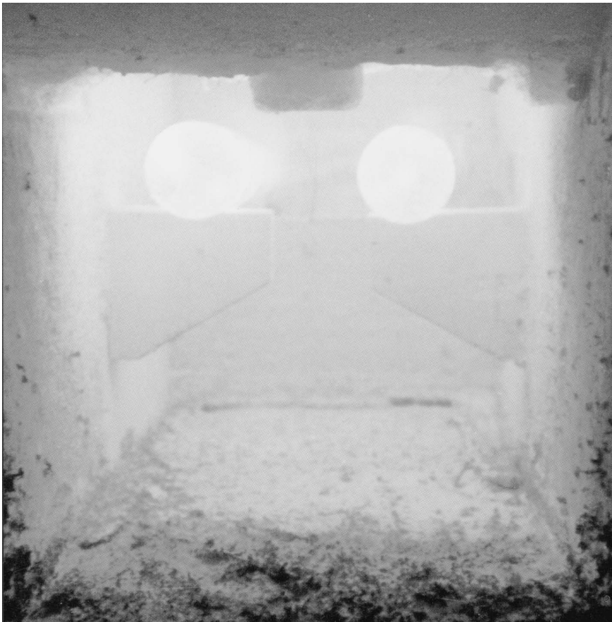
Figure 13.1 Radiant-tube burner schematic (top). Photograph of two radiant-tube burners in an aluminum holding furnace (bottom).
