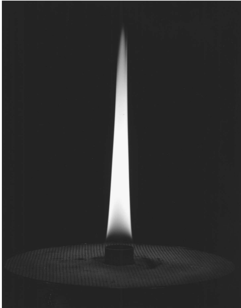
Figure 9.6 Laminar ethylene jet diffusion flame. Note soot “wings” at sides of the flame near the tip.
