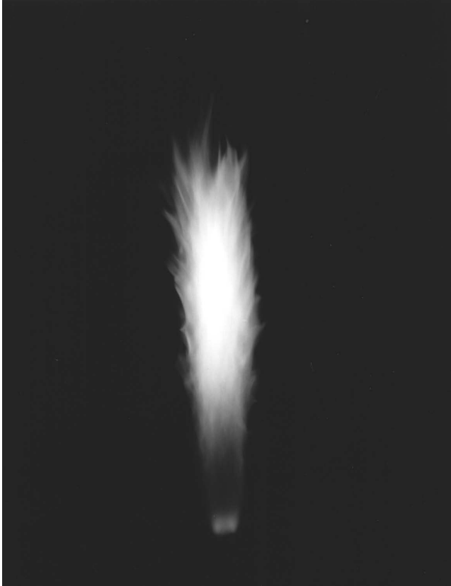
Figure 13.8 Photograph of lifted ethylene–air jet flame ( d_j = 2.18 mm). The base of the lifted flame is wide and appears blue. The burner exit is at the bottom of the frame.
