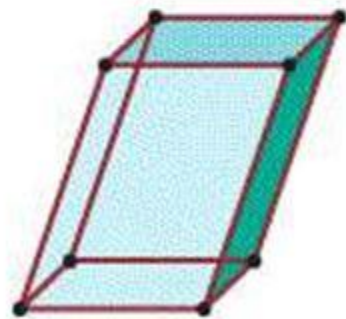
Monoclinic a \neq b \neq c \alpha = \gamma = 90^\circ, \beta \neq 90^\circ
