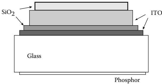
FIGURE 15.19 Glare reduction filter applied to the face of a display. The high index material is made both absorbing and conducting.
