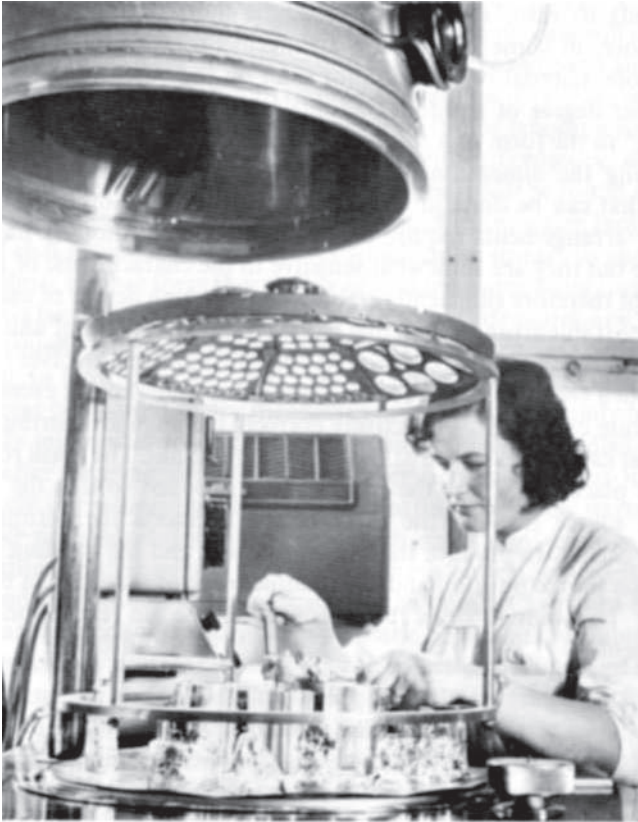
FIGURE 13.5 Interior of a machine with a domed calotte. (Courtesy Balzers AG.)
