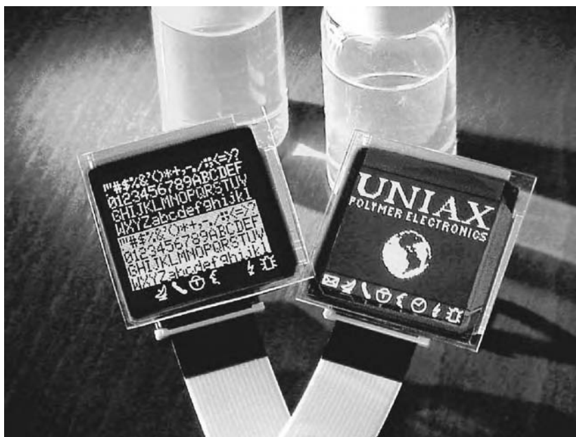
FIGURE 1.24 PM displays in 96 \times 64 format made at DuPont Display.
