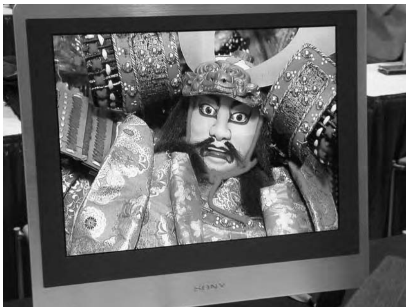
FIGURE 7.12 A 24" AMOLED display fabricated by Sony using top-emission pixel architectures.
