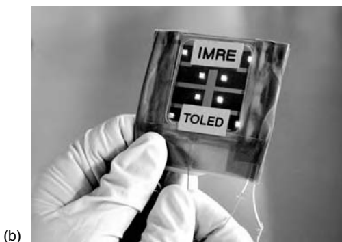
FIGURE 6.15 (a) EL spectra of a set of structurally identical OLEDs having a bilayer anode of metal/ITO. The inset pictures are the actual photographs taken for the microcavity OLEDs demonstrating the color tuning with graded ITO thickness. (b) Top-emitting OLEDs with microcavity architectures to emit variable color and to enhance the light output using single emissive material.
