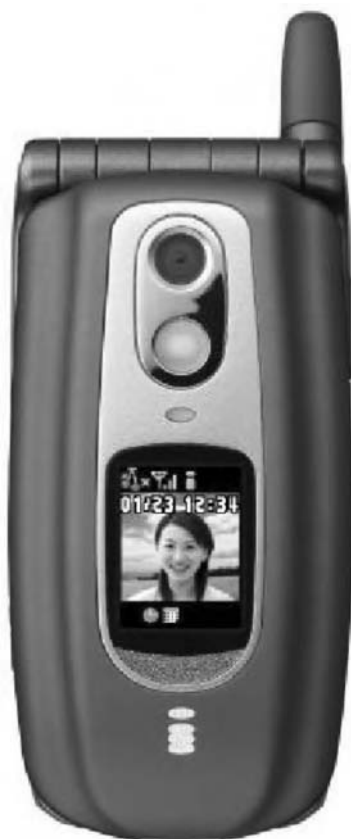
FIGURE 7.15 A commercially available Fujitsu cell phone incorporating a Pioneer manufactured OLED subdisplay that contains both phosphorescent (red) and fluorescent (green and blue) pixels.
