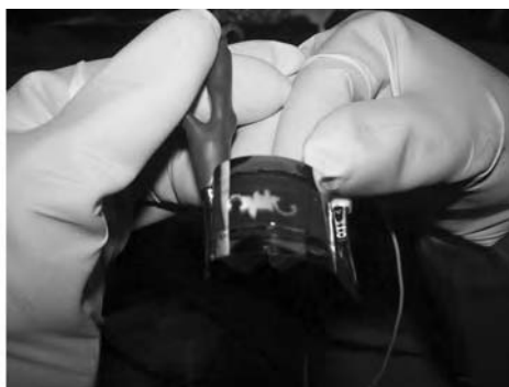
FIGURE 6.24 (a) Luminous efficiency of two top-emitting OLEDs with a configuration of glass/Ag (200 nm)/ITO (130 nm)/PEDOT (80 nm)/Ph-PPV (80 nm)/semitransparent cathode (closed circles), and Al-PET/acrylic layer/Ag (200 nm)/CF x (0.3 nm)/Ph-PPV (110 nm)/semitransparent cathode (open diamonds). (b) A photo image showing a flexible top-emitting electroluminescent device on an Al-PET substrate.
