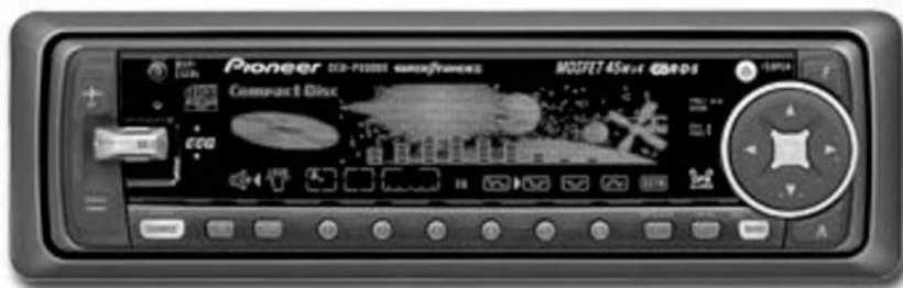
FIGURE 7.2 The world's first commercially available OLED display (1999). The display is manufactured by Pioneer Corporation and is incorporated into automotive stereos.
