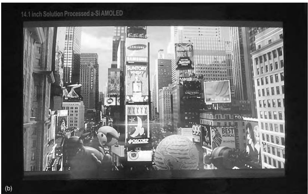
FIGURE 1.25 Photo of a full-color AMOLED in 4" diagonal, QVGA format (a), and 14.1" diagonal WXGA (HDTV) format (b).
