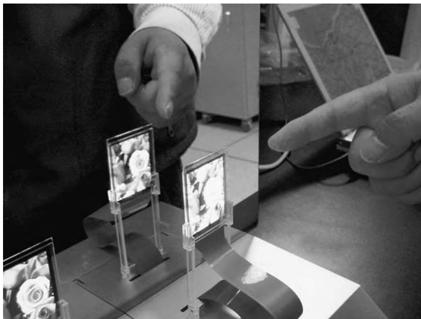
FIGURE 7.13 A 2.2" full-color transparent AMOLED display fabricated by Samsung SDI incorporating phosphorescent dopants.
