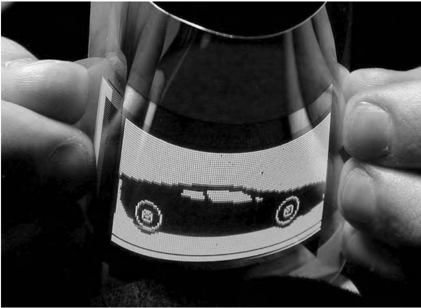
FIGURE 7.17 A 128 \times 64 monochrome PMOLED display on a 175\text{-}\mu\text{m} thick flexible PET substrate. The image is displayed at a luminance of 200\text{ cd/m}^2 .
