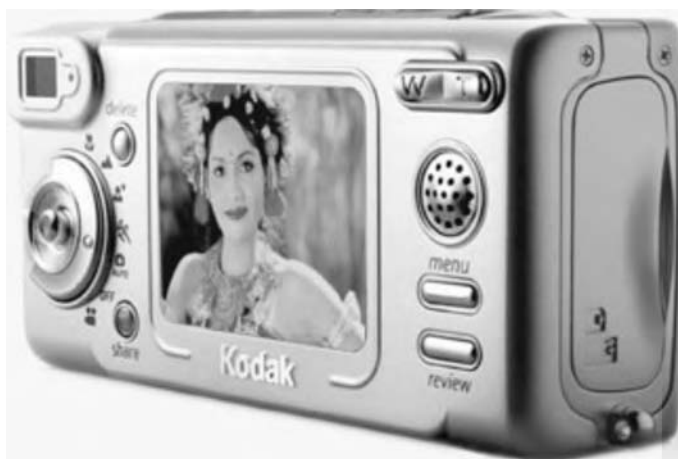
FIGURE 7.16 A commercially available digital camera containing a full-color AMOLED display from Sanyo–Eastman Kodak.
