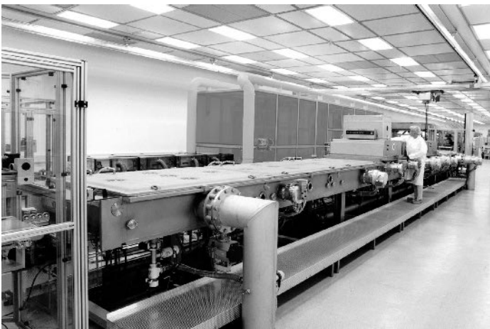
Figure 6.14 Large area in-line sputter coater (Von Ardenne Anlagentechnik, Dresden, Germany) for the deposition of molybdenum and zinc oxide at the Wuerth Solar pilot line in Marbach, Germany. Reproduced with the permission of Von Ardenne Anlagentechnik GmbH.
