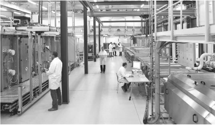
Figure 6.13 Partial view of the pilot production line for CIS modules (substrate size 120 \times 60 \text{ cm}^2 ) at Sulfurcell in Berlin, Germany. Sulfurcell uses the process sequence shown in Figure 6.3. Reproduced with the permission of Dr. Nikolaus Meyer, Hahn-Meitner-Institut Berlin GmbH.
