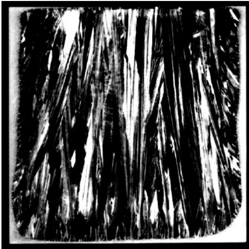
Figure 2.7 Top view of a ZMR recrystallized layer on a 50 \times 50 \text{ mm}^2 \text{SiO}_2 coated mc-silicon substrate. Scan direction was from bottom to top, the molten zone was in the horizontal direction. Images taken from C. Hebling, Die kristalline Silicium-Dünnschichtsolarzelle auf isolierenden Substraten, Ph.D thesis, Universität Konstanz (1998).
