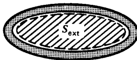
Figure 11.13 The “external” self-inductance of a loop is often calculated by calculating the flux through the area external to the wire (shaded area) to avoid possible divergences at the wire itself.
