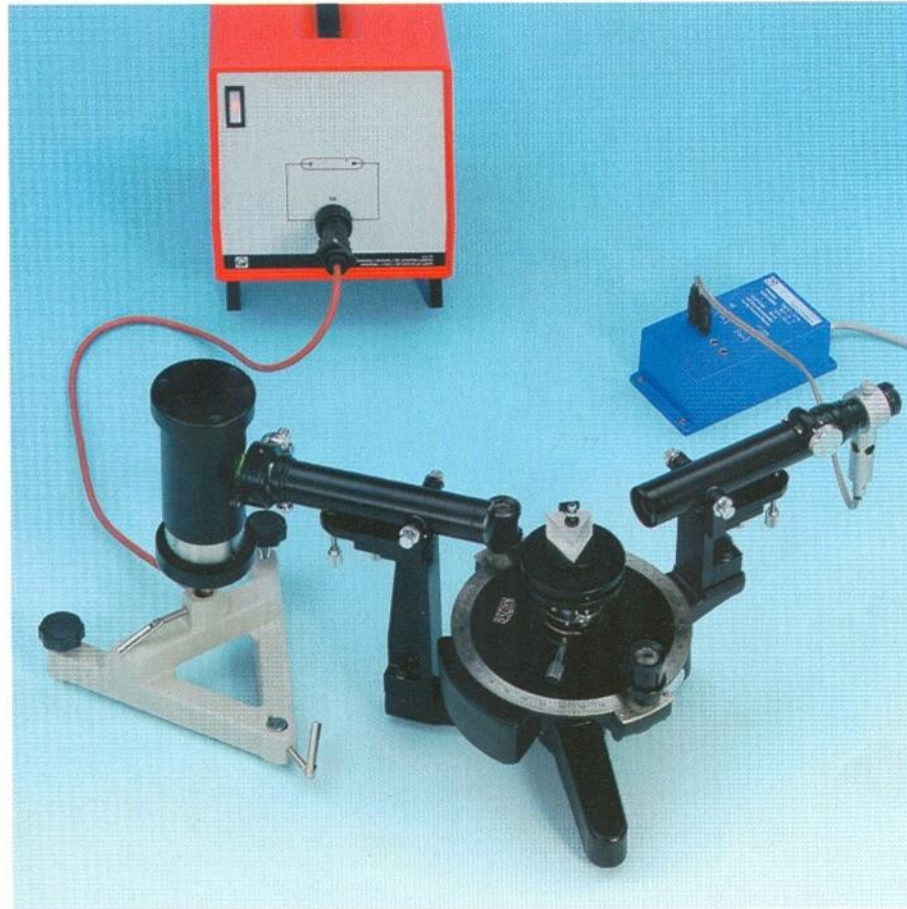
Measuring the line spectra of inert gases and metal vapors using a prism spectrometer
