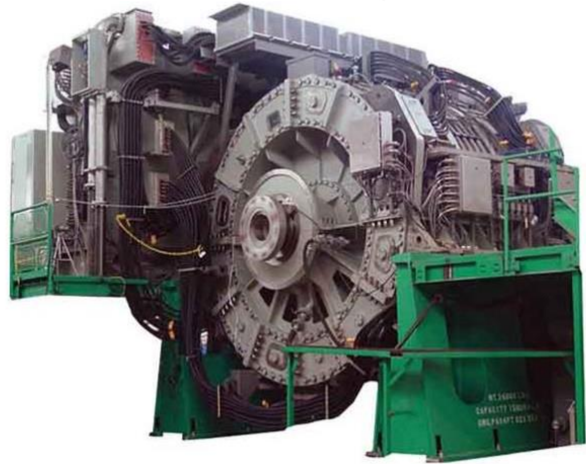
Fig. 2. DRS' 36MW permanent magnet propulsion motor and variable frequency drive.
