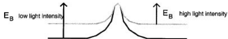
Fig. 8.22. Grain boundary height at different light intensities. At high light intensity, changes in the charge stored in the interface states reduce the height of the potential barrier.
