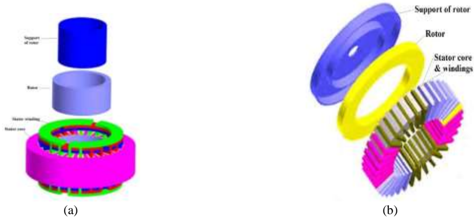
Figure 1. Structure of various types of hysteresis motor: (a) Circumferential-flux (b) Axial-flux
