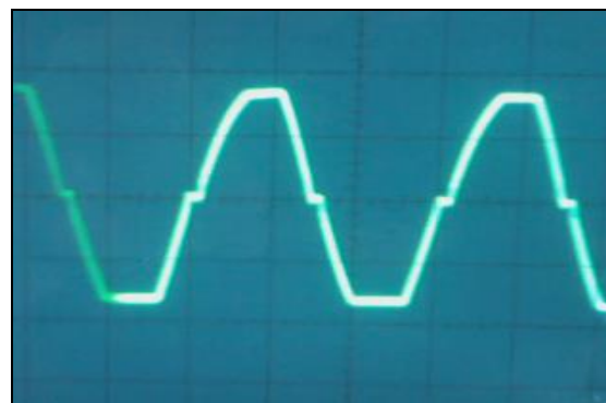
Fig. 14: Filtered Output Voltage.
