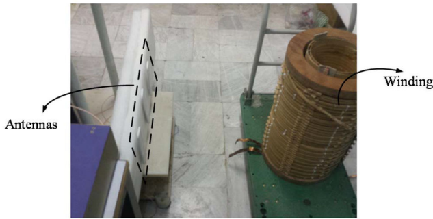
Fig. 4 Schematic of single-phase winding and antennas
